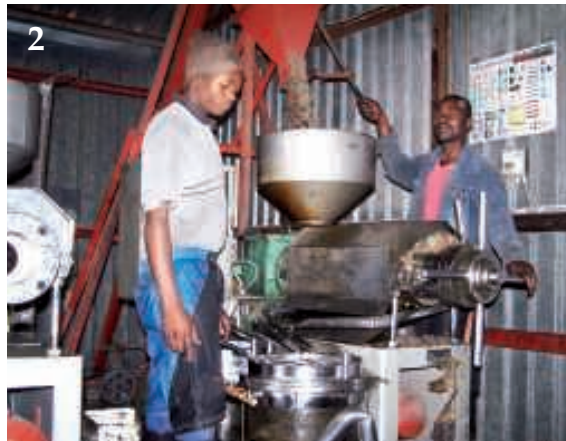
1. Louis Claassen at the oil pressing plant. 2. Labourers Joseph (left) and Sipho (right) feed sunflower into the oil press. The plant is not very labour intensive and doesn't require much direct employment. MacDonald says when farmers produce their own biodiesel their input costs decrease significantly. This enable farmers to utilise marginal land for production, which in turn necessitate increased labour. 3. Unclean oil still to pass through the filter press.
